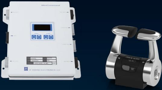
MiniCommand is the evolution of standard electronic controls. MiniCommand provides affordable single or twin lever control of electronically actuated diesel engines and marine transmissions. Designed specifically for pleasure craft and light duty commercial applications up to 60 feet in length, with a maximum of two control stations, the MiniCommand control processor incorporates the logic circuits for two engines and transmissions in one compact package.
